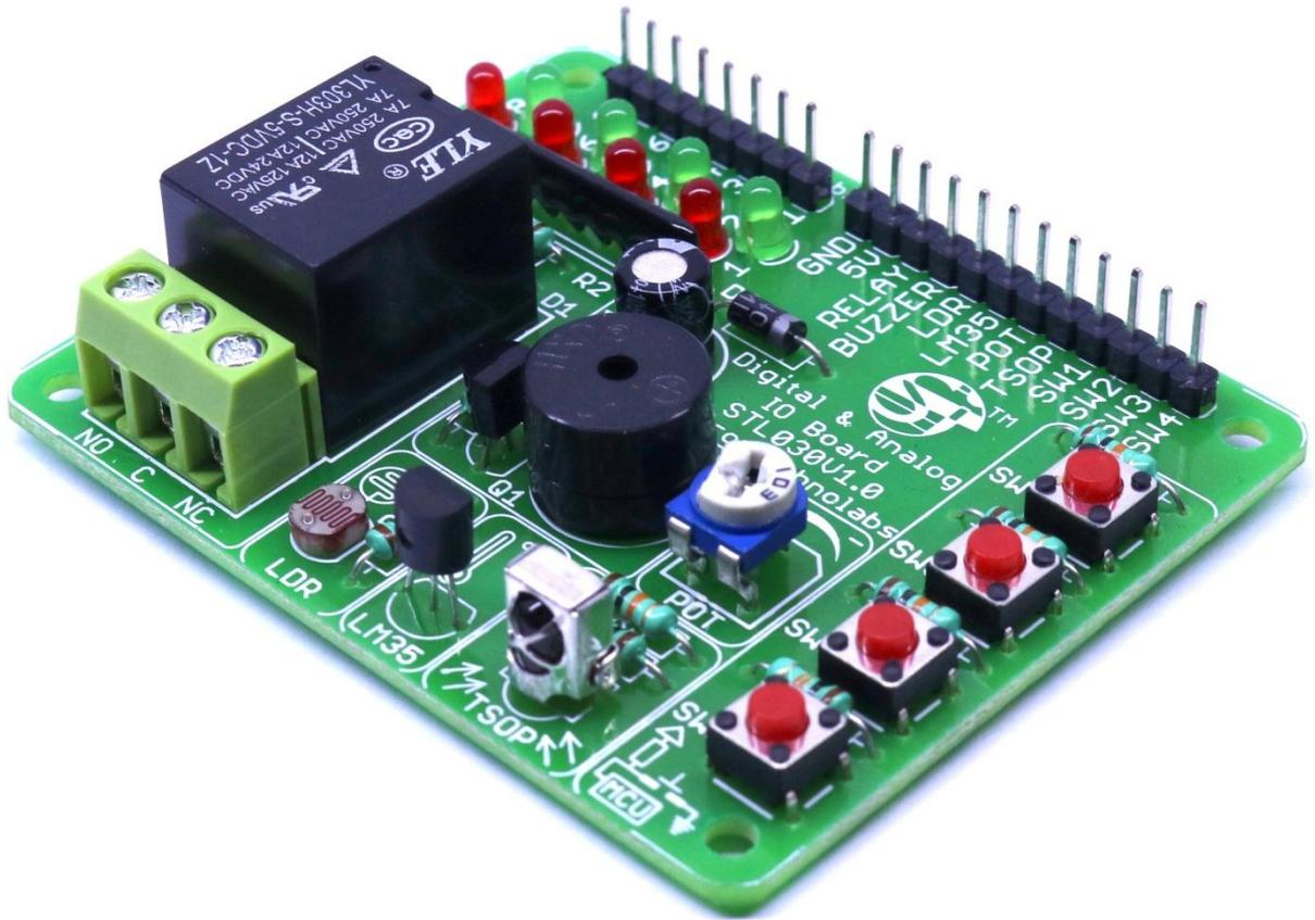
Digital & Analog IO Breakout Board
