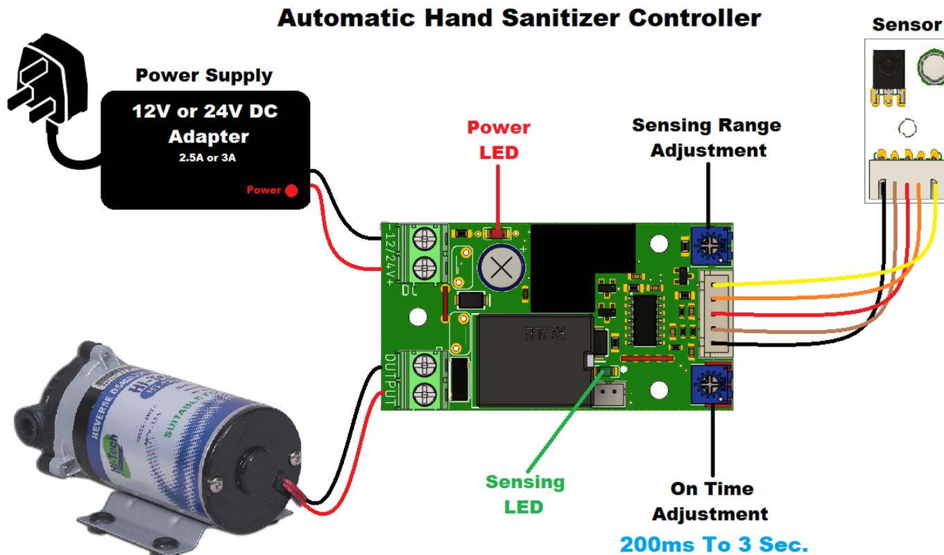
Note: Power Adapter and Pump are for illustration purpose only not including with controller.
